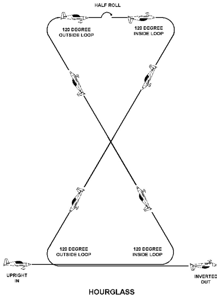
From level flight perform a 1/3 inside loop through approximately 120 degrees to inverted 60 degree climb. At the top of the climb perform a 1/3 outside loop to level flight. Half roll to inverted. Perform a 1/3 inside loop through approximately 120 degrees to upright 60 degree dive. Perform a 1/3 outside loop through approximately 120 degrees to level flight, exit inverted.
